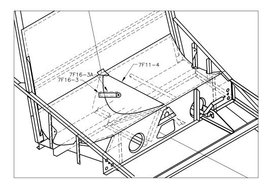
The Central Seat Belt Doubler 7F16-3A is placed inside the Tunnel 7F11-4 to double the Central Seat Belt Attachment 7F16-3 using 5 rivets A5.
