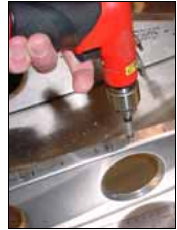
Pre-drill the rib flange with #40 pilot holes.
