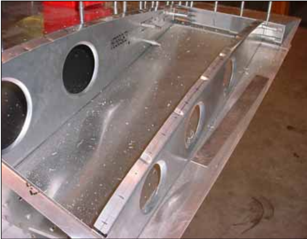
Pre-drill the rib flange with #40 pilot holes.
