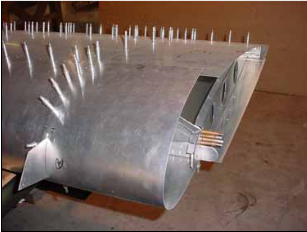
Top view of the leading edge (nose skin) 7V7-1. The leading edge skin will be trimmed to make the connection to the root nose rib.
