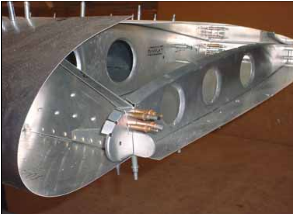
Detail to show the root nose rib 7V4-1
