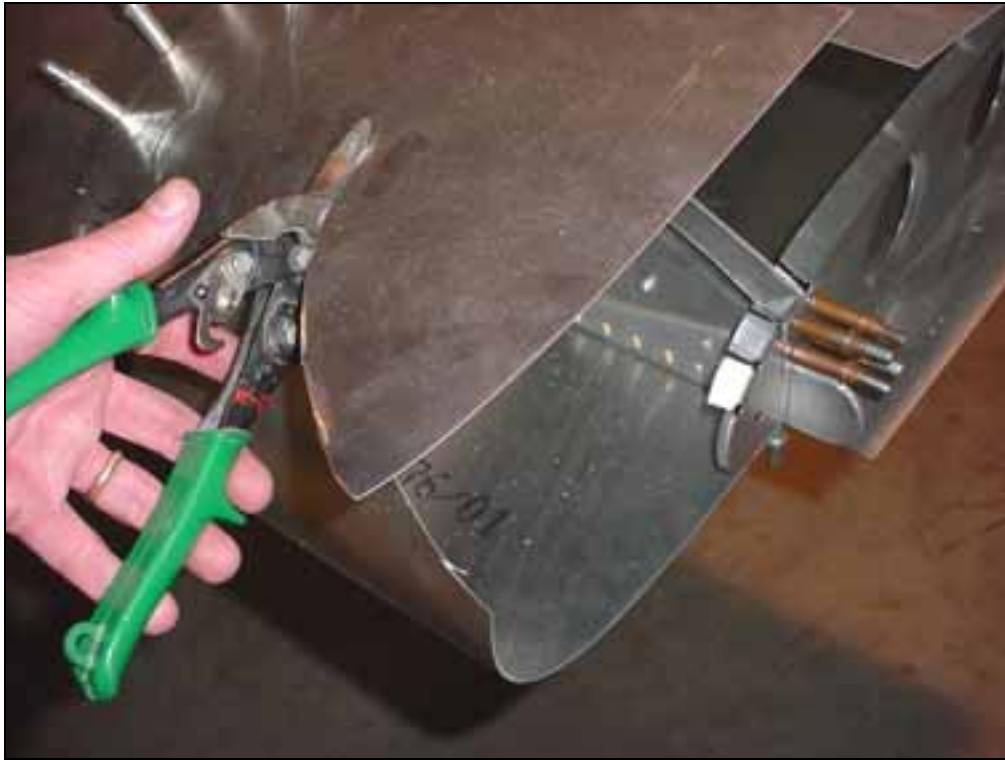
Rough cut the nose skin 7V7-1 (top side inboard or nose rib #1)
