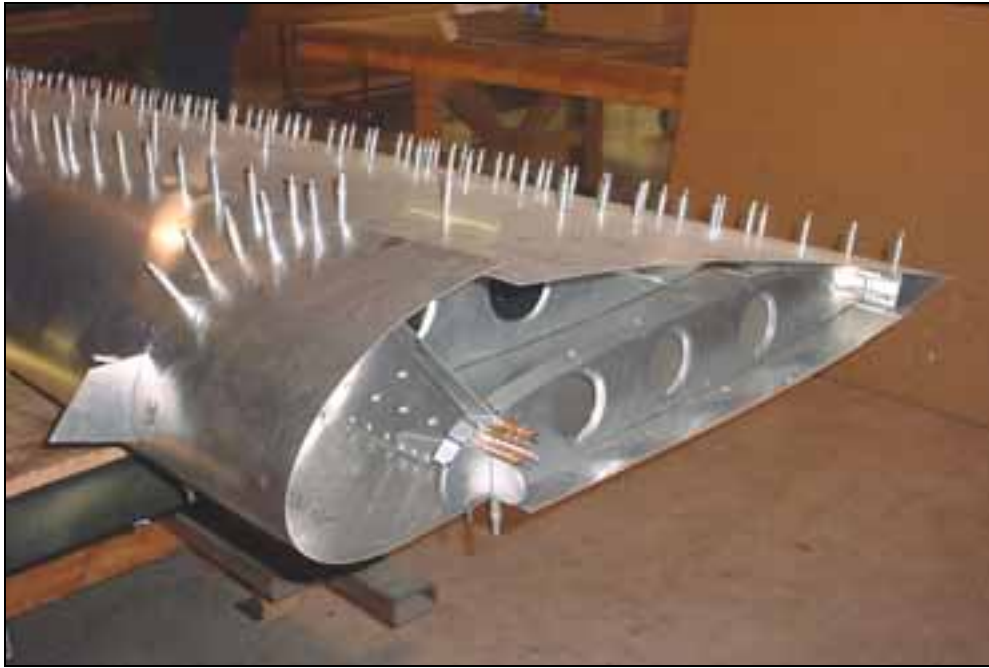
I/B end of right wing, before the skins are trimmed.
