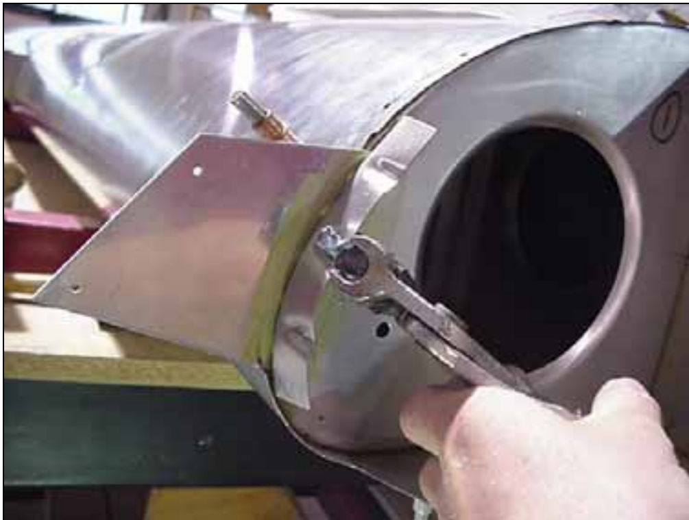
Also crimp the bent L angle riveted to the side of the nose rib.
