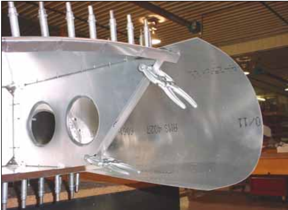
L angle overlaps behind the top and bottom angles 7V8-2 and 7V8-3.
