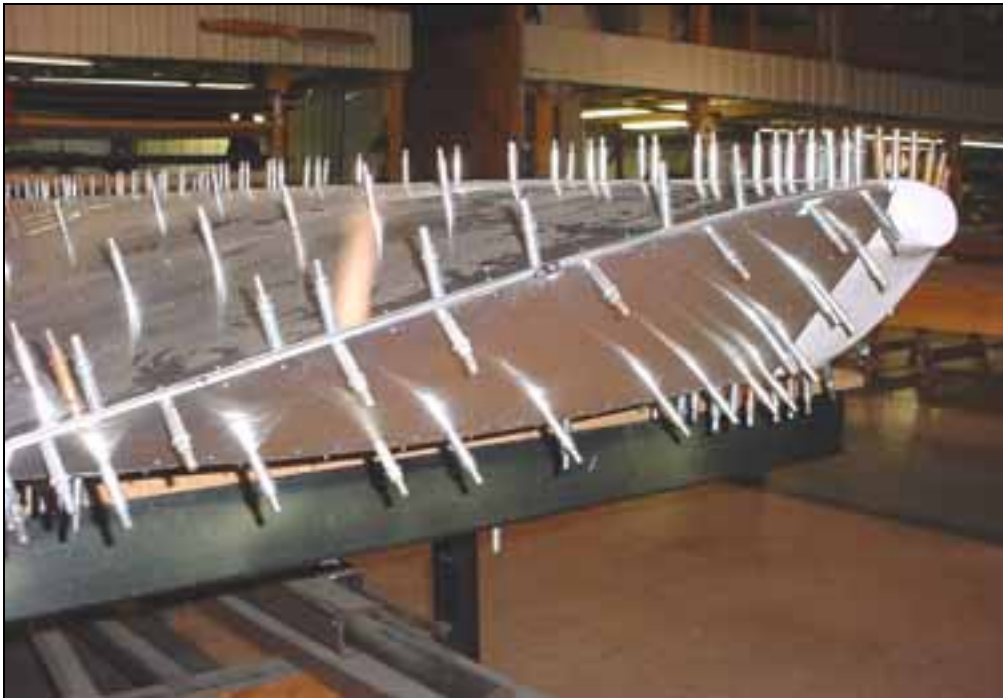
Drill and Cleco
