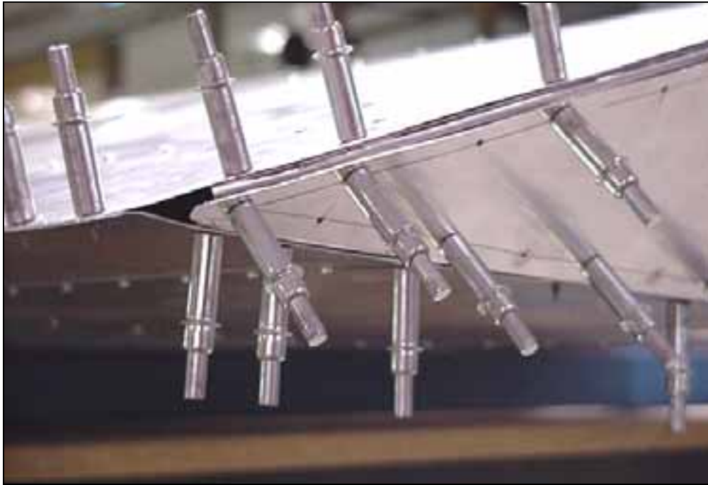
Detail of the trailing edge: rear part of the skin.
