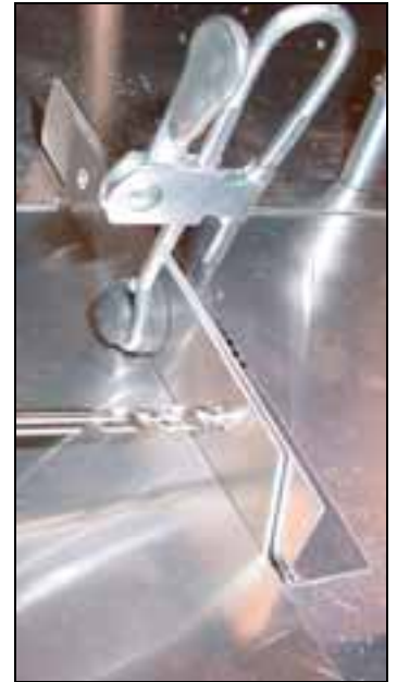
Back drill through the #20 in the bracket.
