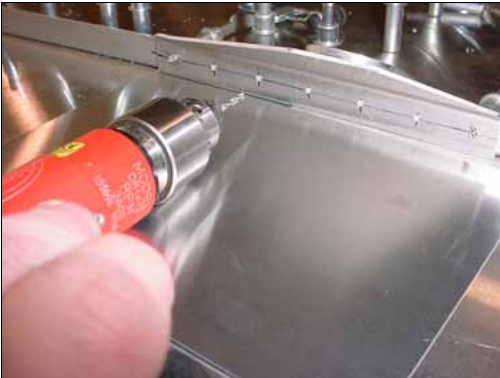
Photo of the outboard side of the doubler 7V8-1SP
