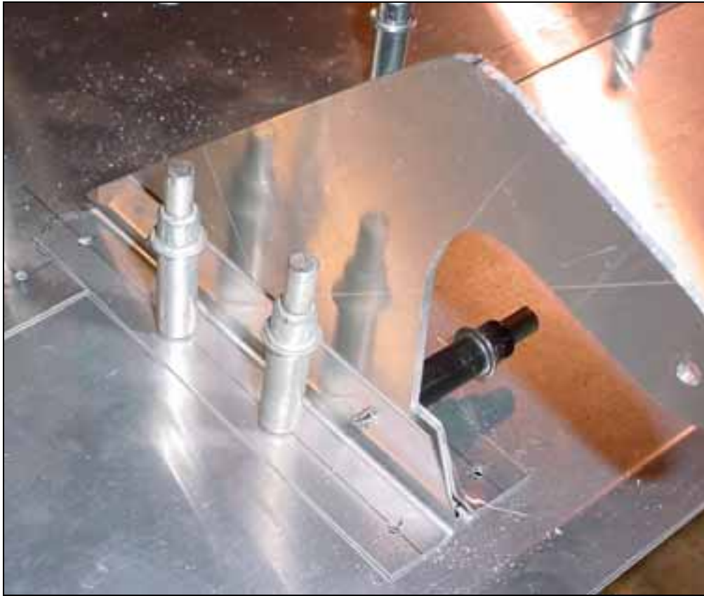
Trim the ends of the L angles.
