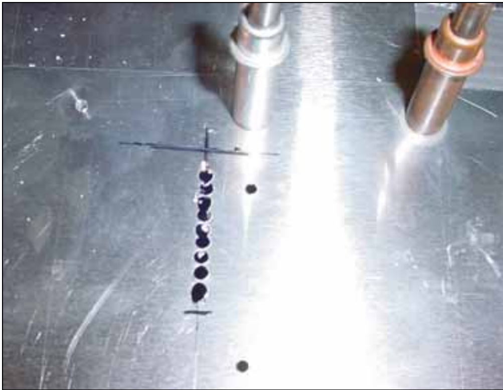
Filled slot. Re-install the nose rib.
