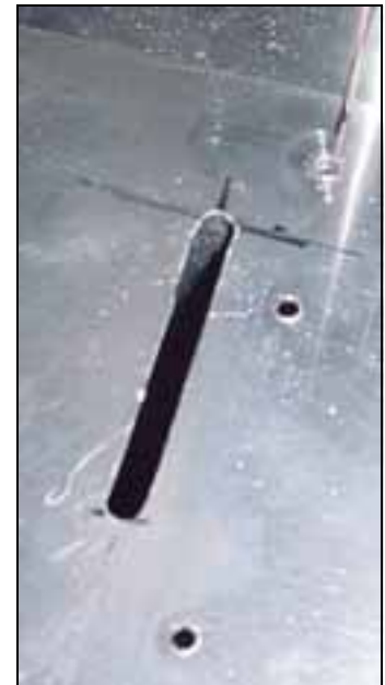
Filled slot. Re-install the nose rib.
