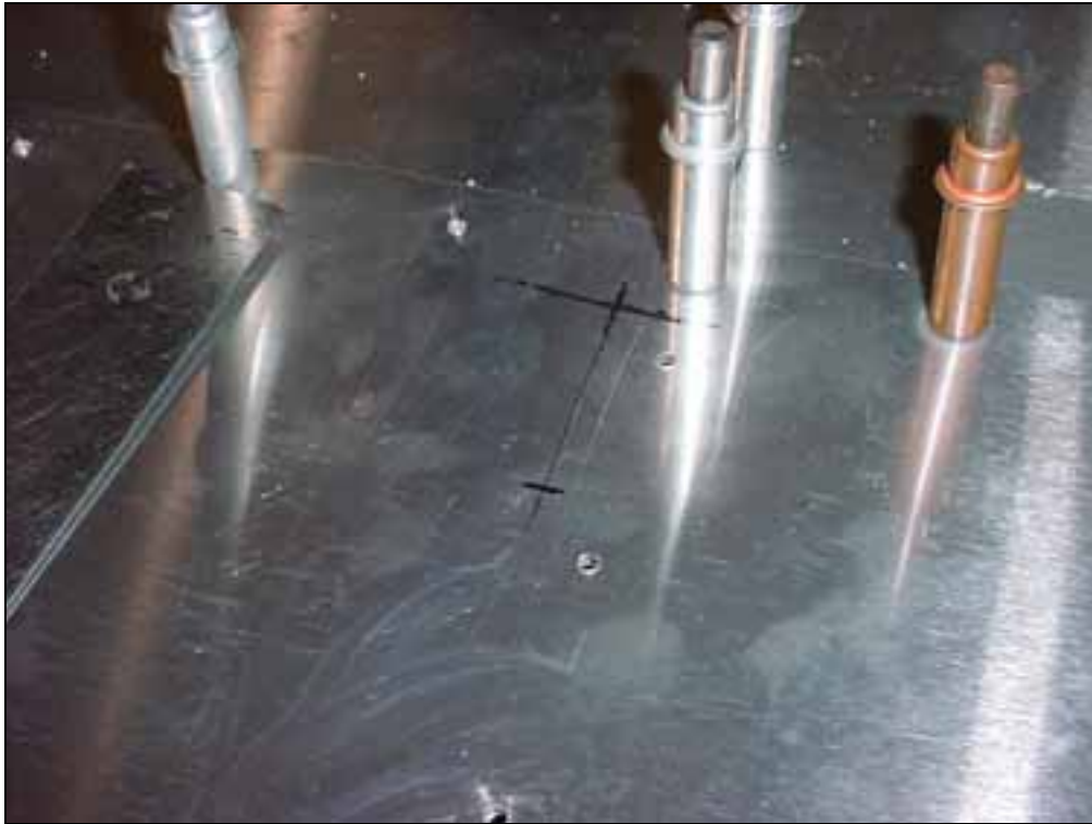
Cutout on the I/B side of nose rib #5
