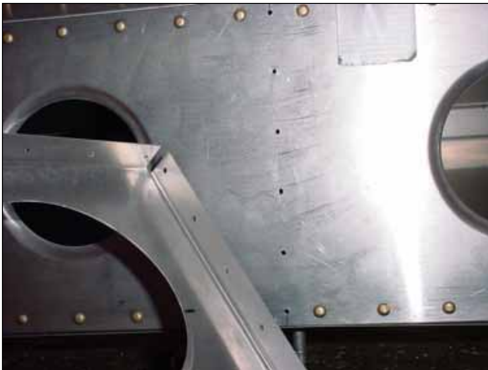
Check to make sure the location of the cutout is in front of the spar.
