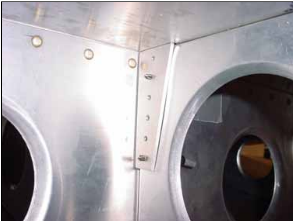
Drill and cleco 6 RIVETS A5 Ref. bottom diagram on drawing 7-V-8
