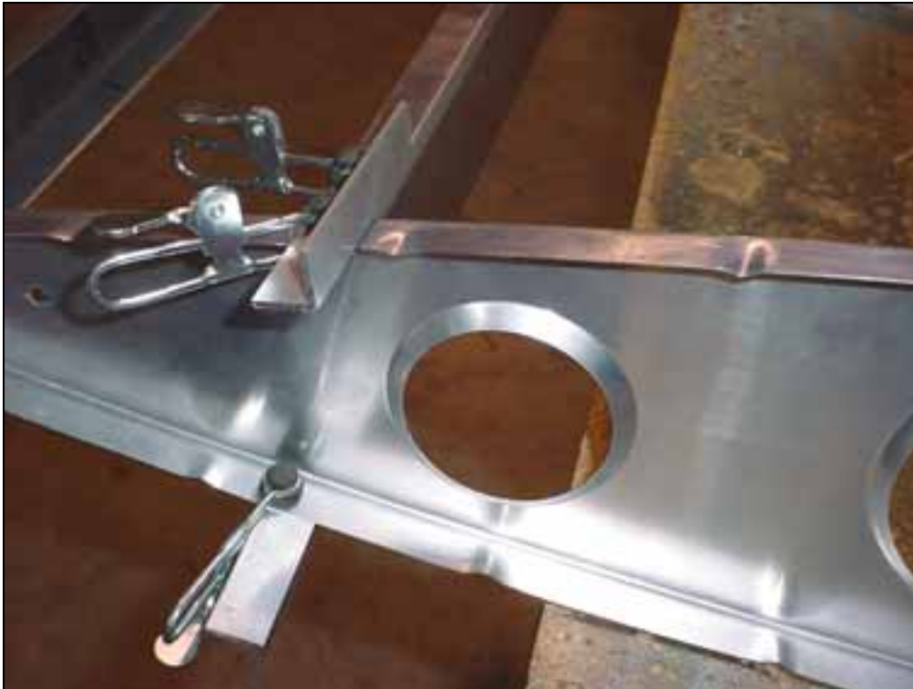
The channel fits inside the inboard rib.
