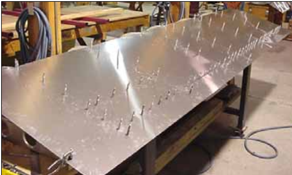
Finish drilling the skin to the ribs and channels.
