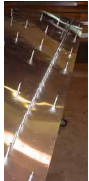
Rivet line through channel.
