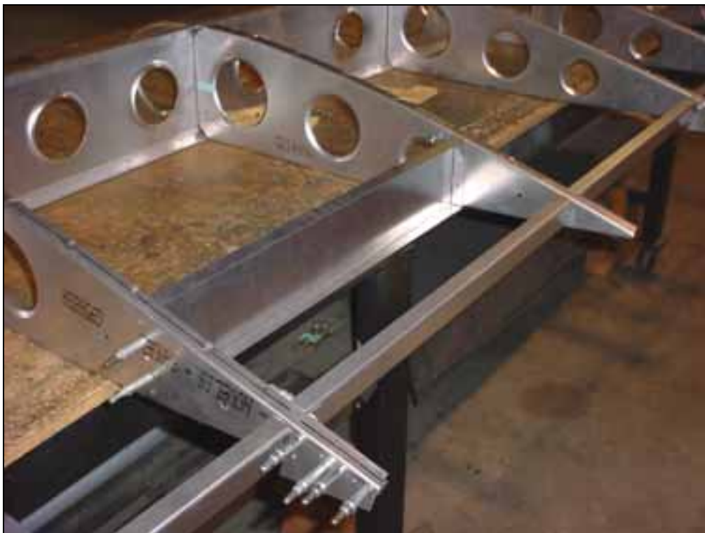
Clamp the extrusion to the rib flange.
