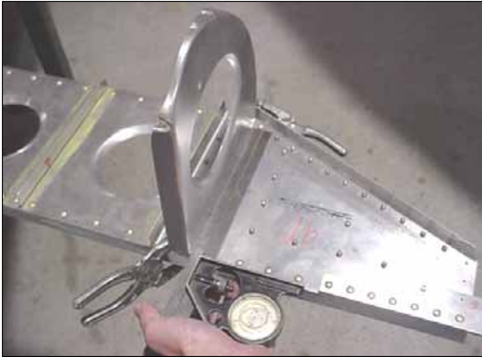
Mark rivet line on the back side of the spar flange of each nose rib. RIB ORIENTATION: All ribs are positioned with the flanges pointing towards the outboard wing tip.
