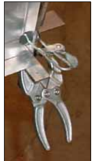
First clamp the bottom flange of the rib to the bottom extrusion. Then clamp the rib to the spar.
