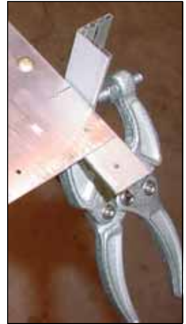
Clamp a piece of extrusion or other piece of flat plate to the bottom flange of the spar (centered on the rib rivet line).
