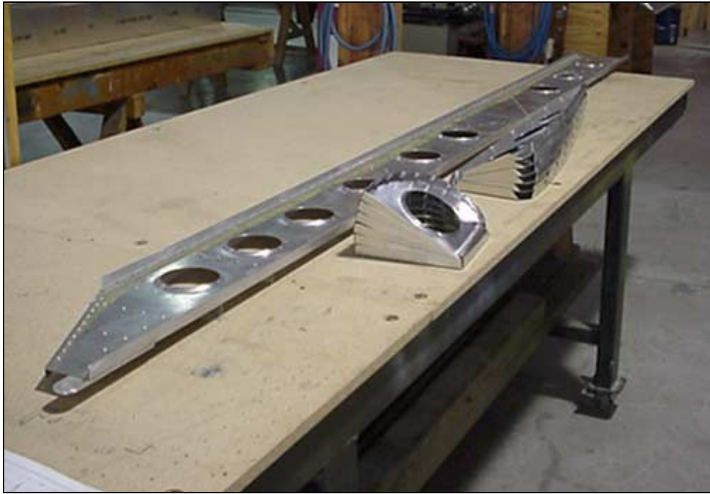
Building the right wing skeleton.
