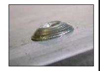
**CHECK** that there is no gap between edge of rivet head and sheet
