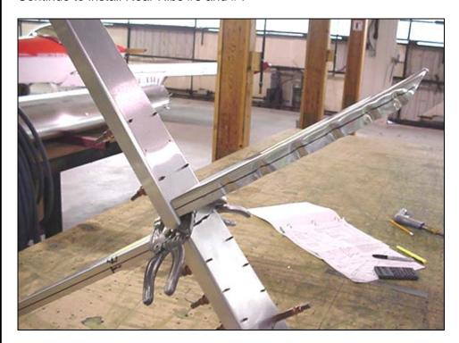
CHECK: Rib is centered left and right on the Spar. This can be done by clamping pieces of extrusion to the side flanges of the Nose Rib before clamping the Nose Rib to the Spar (not shown in photo).
