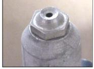
**IMPORTANT**: use the special machined riveter nose piece to rivet.
