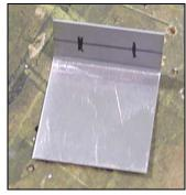
Mark and drill 2 holes #30 in the short flange (8mm edge distance.
