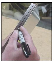
Layout flange center line on ribs 2, 3 and 4
