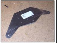
or 75R2-4 Horn 7R1-1 Rudder Bottom Rib #1 or 75R1-1 Rudder Bottom Rib #1
