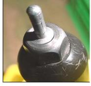
The diameter of machined nose piece is the same diameter as the rivet head
