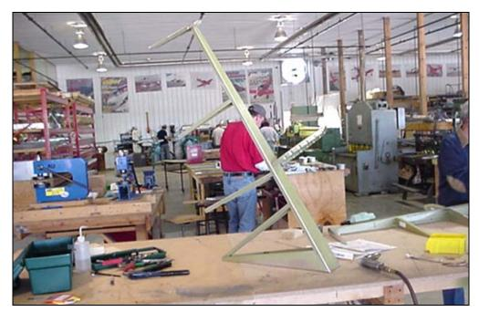
**Rudder Skeleton** (when riveting, the rivet head is installed on the front side of spar).
