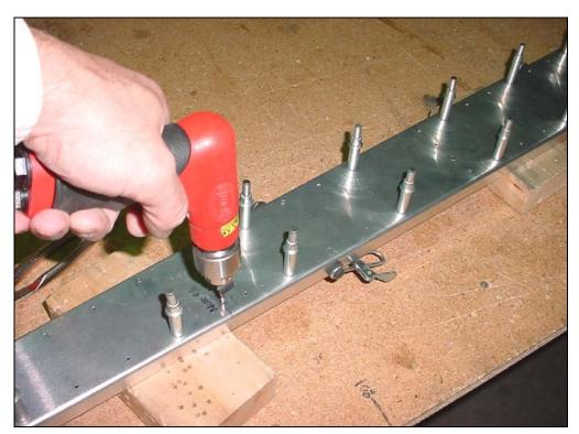
Support the spar on wood blocks. Drill and cleco the Spar Doublers to the Spar at every other hole, then drill the remaining holes without adding more clecos for A4 rivets.
