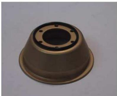
1 Reference photo of o-ring on wheel half prior to installation. The radius area just outside the bolt circle should be inspected for nicks or scratches. Any nicks or scratches found should be polished smooth as they can provide a leak path around the o-ring when in the final seated position
