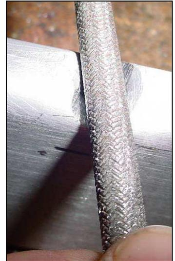
**CHECK:** The notch is not too tight: taper the sides of the notch to allow the gear to flex around the welded gear bolts.
