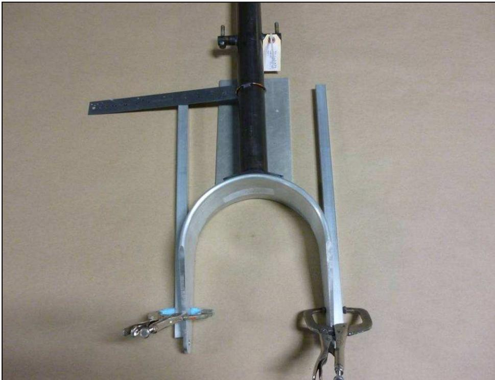
Center the Nose Gear Strut Assembly on the Wheel Fork Doubler and Wheel Fork.
