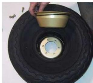
5 Insert wheel half with o-ring into tire and mate with opposite half. O-ring is still installed on bead seat.
