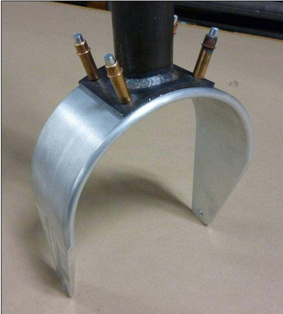
**7L1-1J Nose Gear Strut Assembly**
