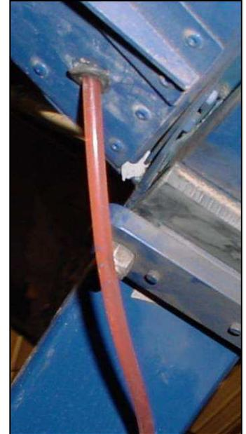
Location of grommet in cabin floor, see bottom left diagram on drawing 7-F-9
