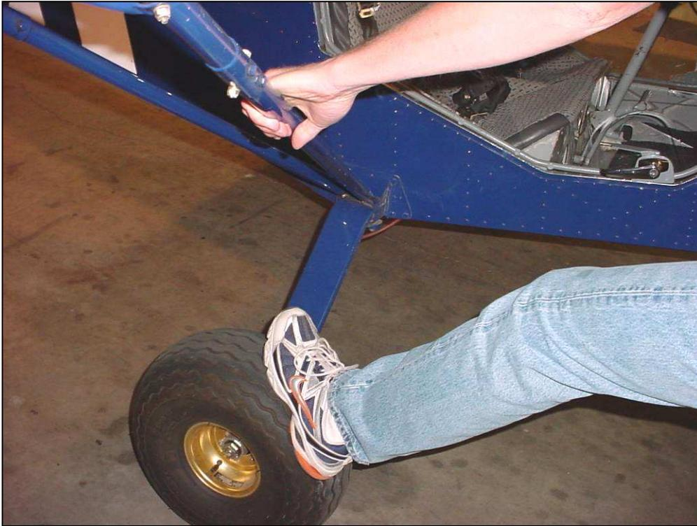
Check the gear is not loose: hold the aircraft by the wing strut, place a foot on the wheel: hold the aircraft from moving as you try to turn the wheel. Check both wheels.
