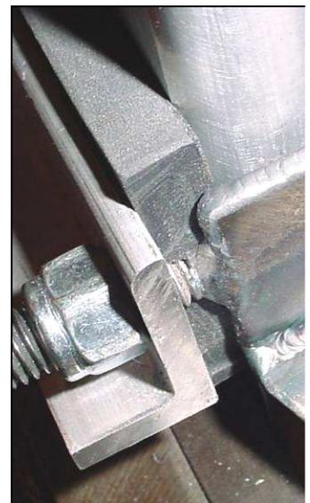
Check that the Gear Plate does not make contact with the Channel Pick (bottom of gear strut fitting).
