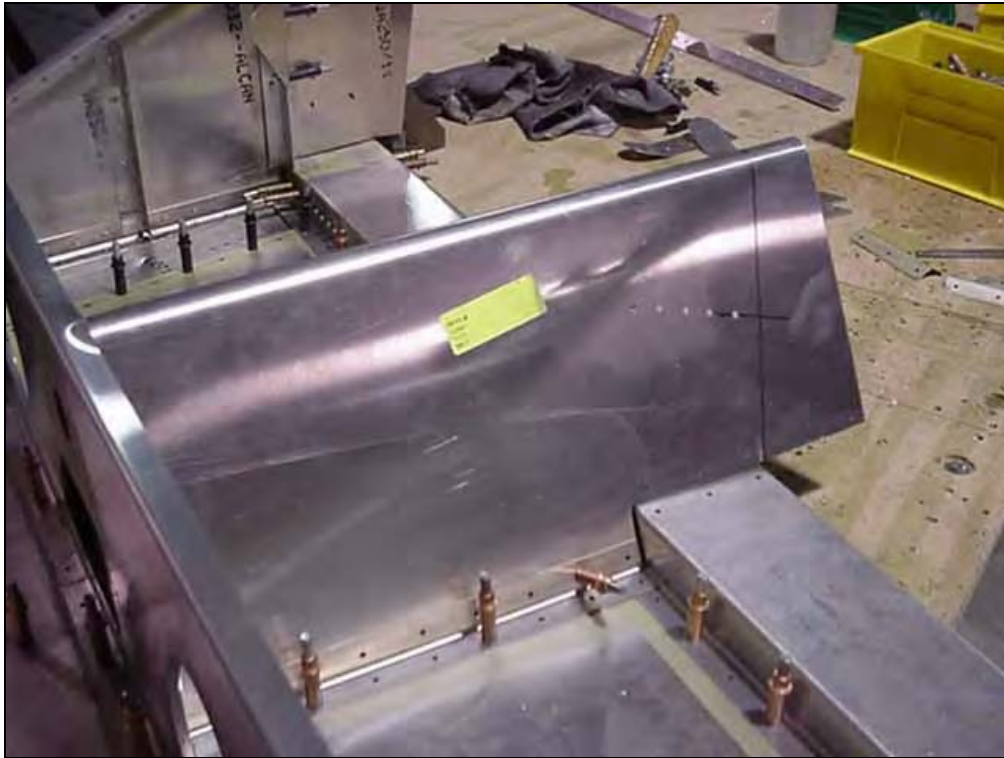
7F11-4 Tunnel 7F11-4A Tunnel Angles
