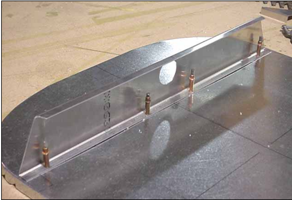
7F7-1SP Upper Channel 7F1-1 Firewall
