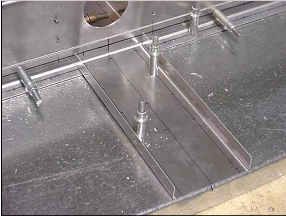
7F7-3 Vertical Top Channel 7F1-1 Firewall
