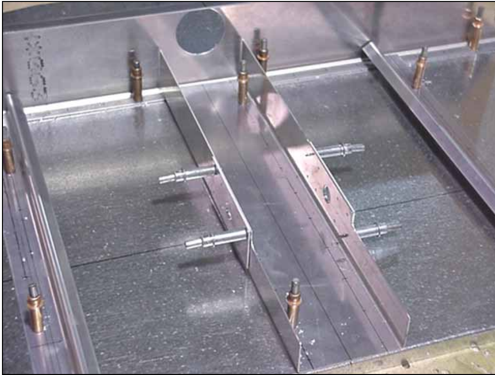
7F7-2C Vertical Lower Channel 7F1-1 Firewall
