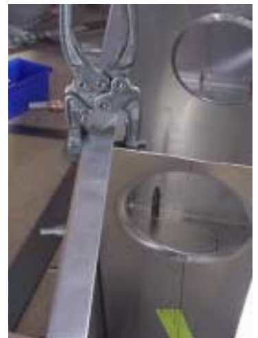
Clamp the Rear Tail Frame to the Side Skin. Line up the Tail Frame with the predrilled holes.
