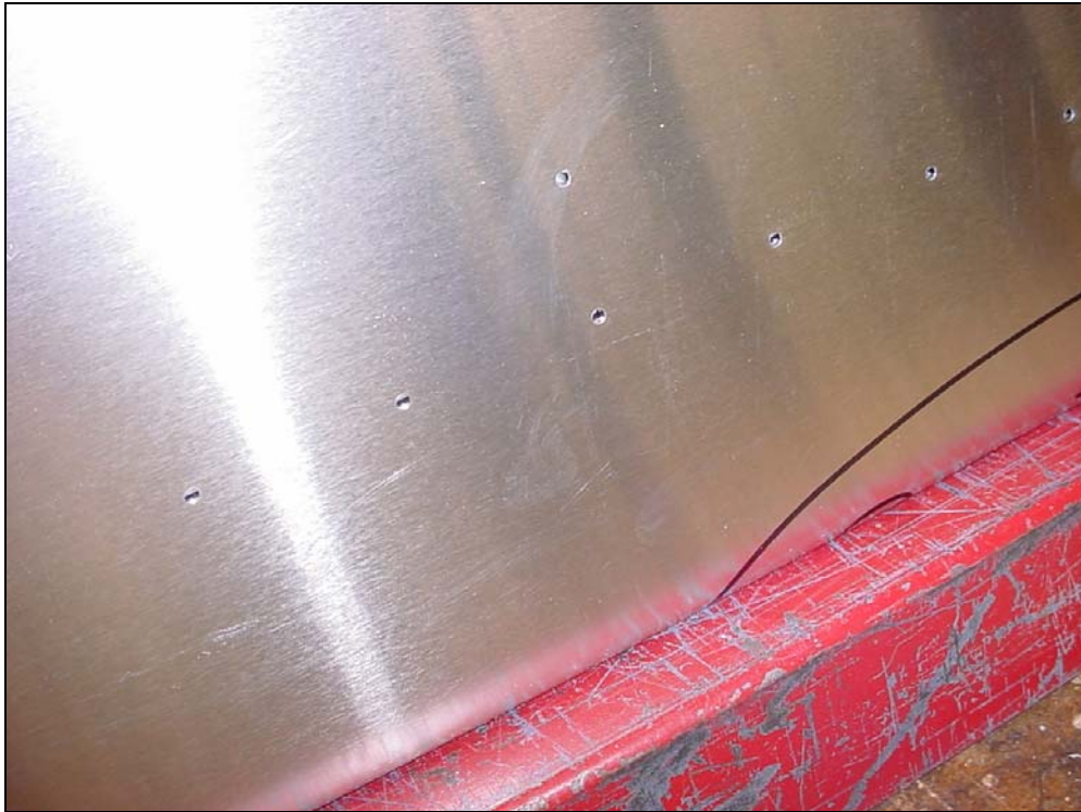
Rivet line visible through the pilot holes.
